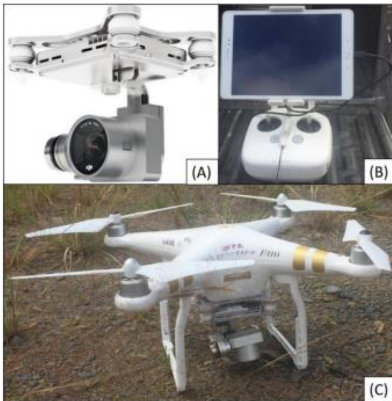
Figura 3 - Câmera (A), controle com tablet (B) e o VANT Phantom 3 Professional (C)
